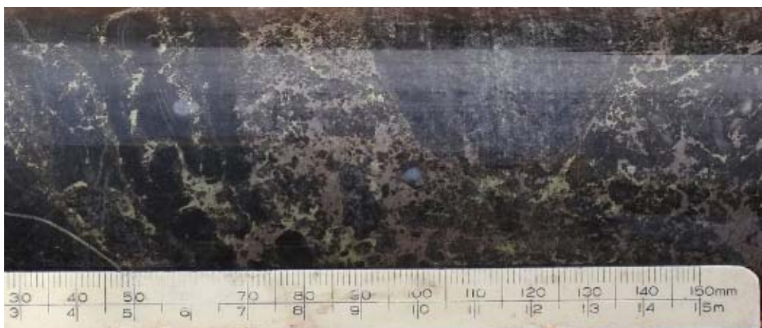
Figure 3: Breccia Matrix Mineralisation in gabbro (Hole ASPDD2, interval 45.4m)
